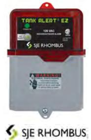
Interlocking enclosure features unique sound chamber to amplify the horn while helping prevent moisture from entering. Once the condition is cleared, the alarm automatically resets. Standard features include an alarm test/silence switch, green power on indicator, and auxiliary contacts for remote devices.
