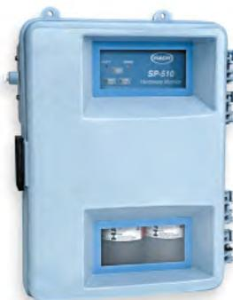
Alarm point is 2 ppm (expressed as mg/L of CaCO<sub>3</sub>) and is selected by choosing the appropriate model. A rugged, corrosion-resistant and shatterproof ABS plastic case protects the analyzer and reagents. The sealed case is IP62-rated and has a hinged door for easy access to internal components. Easy-to-read LED indicators show a simple "HARD" or "SOFT" sample status. Use the built-in alarm relay to actuate an external annunciator.
