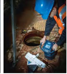
The FLO-DAR® AV Sensor offers an optimal solution for non-contact, maintenance-free monitoring of sewer flow, suitable for both portable and permanent installations.
