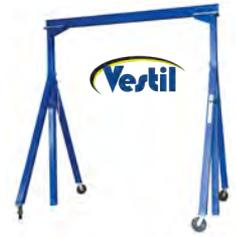
Select from fixed- or adjustable-height gantry cranes. Fixed-height cranes are ideal when there is no need to change the overall height of the unit. Change the height available under the I-beam on the adjustable-height cranes to accommodate various applications. It requires assistance from fork truck or other overhead lifting device to set up.
