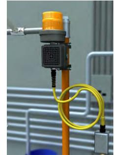
Use NEMA-4X unit (400206) in areas where corrosive materials and caustic cleaners such as disinfectants are used. Class I, Division 2 unit (400207) is ideal for use in C1D2 hazardous environments where flammable liquids or gases are not present during normal operating conditions. All units require 120 VAC, 0.3 amp electrical supply.
