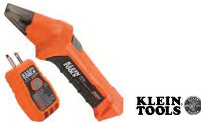
Quickly and accurately locate the correct circuit breaker in a panel to which an electrical outlet or fixture is connected. The ET310 Circuit Breaker Finder with Integrated GFCI Outlet Tester combines a digital circuit breaker finder and a GFCI outlet tester in one tester set. The transmitter is connected to the electrical outlet or fixture in the circuit while the receiver is used to scan the breakers in the circuit panel. The Transmitter also works as a GFCI outlet tester.
