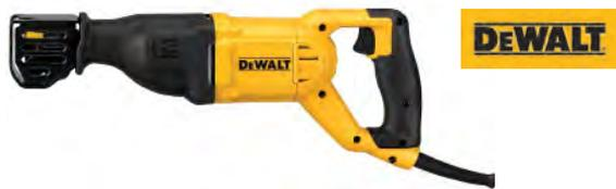
The Reciprocating Saw has a powerful 12 amp motor with a variable-speed trigger that provides up to 2900 strokes/minute with a 1-1/8" stroke length for fast cutting. Use the four-position blade clamp for flush cutting and increased versatility. A keyless, lever-action blade clamp offers quick and easy blade changes.
