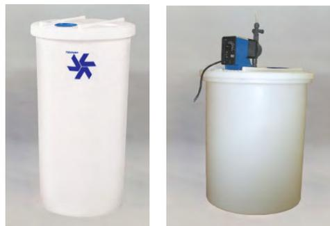
These tapered HDPE Chemical Solution Tanks feature rigid covers that accommodate top mounting of CHEM-TECH 100, 200, most PULSAtron pump models and 1/20-hp flange mount mixers. The covers feature a 4.5" refill cap, 1.4" cap pump accessories and two 3.5" indent for mounting accessories. Tanks are translucent and come with 5-gallon graduations.
