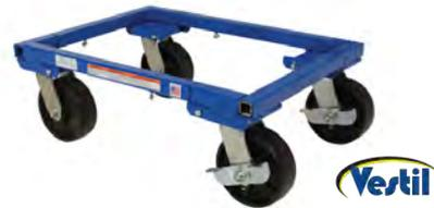
The unique design of the Adjustable Tote Dolly allows both width and length to be changed for use with different size totes. Simply loosen the screws and slide each side in or out to change the size. Welded steel construction with powder-coat blue finish offers maximum durability. Usable length is from 22 to 34"; usable width is from 16 to 24".
