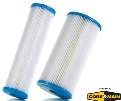
Durable Polyester Pleated Cartridges are durable, washable and reusable. The polyester media pleated around a polypropylene core provide added strength. The ends are immersed in a thermosetting vinyl plastisol which fuses the three components together forming a unified end cap and gasket. The pleated cartridges are bacteria and chemical resistant and provide great dirt holding capacity to extend the time between cartridge change outs.
