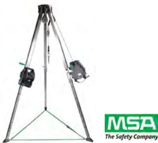
The MSA Workman CSE Tripod Kit provides simple ordering with all the necessary components for a complete safety system. Use the kit to help protect workers in tight spaces. The entire Workman CSE kit takes only minutes to set up; no tools are needed. Kits are ideal for applications in tanks, manholes and other vertical entry work practices.
