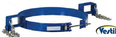
Transport your steel drums easily and safely with the Vestil Tilting Drum Ring. To use, slip the band over the belly of the steel drum and tighten the lock to secure the band around the belly of the drum. Two fork openings each measuring 5-1/4"W x 2-7/8"H accept forks to easily lift the drum.
