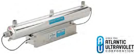
Ultraviolet technology does not rely on dangerous chemicals or heat for disinfection, making this method relatively simple, inexpensive and low maintenance. Ultraviolet purifiers utilize germicidal lamps that are designed and calculated to produce a certain dosage of ultraviolet (usually at least 16,000  $\mu\text{W}/\text{cm}^2$  but many units actually have a much higher dosage).
