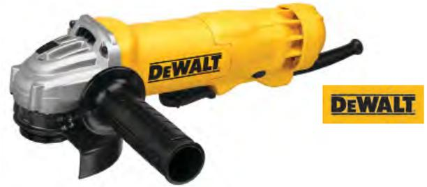
DeWALT 4-1/2" (115 mm) Heavy-Duty, Small Angle Grinder with a powerful 11 amp AC/DC, 11,000 rpm motor provides the best power to weight/size ratio available. A unique dust ejection system ejects damaging dust and debris particles that enter the tool. One-Touch™ guard allows the guard to rotate 360-degrees; Quick-Change™ wheel release offers easy wheel removal.
