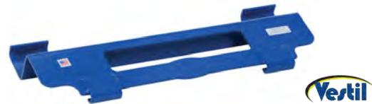
The Non-Adjustable Pallet Jockey is a simple device that allows drivers and warehouse personnel to unload sideways pallets efficiently and safely with their walkie pallet trucks. This unit is ideal for warehouse distribution centers that use one particular electric pallet truck model. To use, simply place the pallet jockey hooks into the fork wheel openings. Fits most popular sizes of walkie truck.
