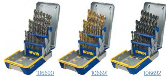
The M35 Cobalt Alloy Steel is a hard, heat- and wear-resistant metal that is ideal for drilling hard and abrasive materials. Each bit features 135-degree split point tips that start on contact and stays on work surface. Bits larger than 3/8" have a reduced shank so you can use the larger drill bits in a standard 3/8" chuck. The included case has removable cartridges to carry bits from case to work site safely.
