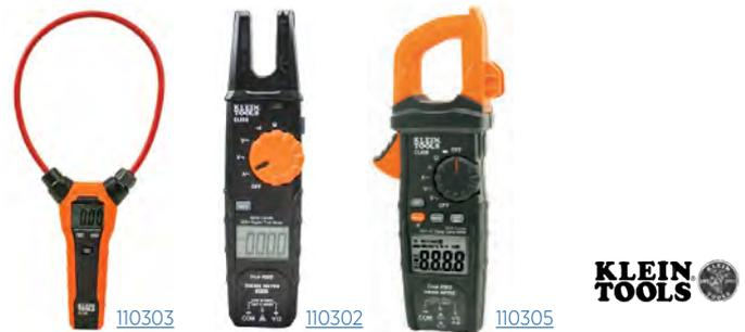
These Auto-Ranging True RMS Clamp Meters provide excellent accuracy and easy-to-read results to help you get your job done. These meters are built to stand up to tough jobsite conditions and have been designed with specific trades in mind.
