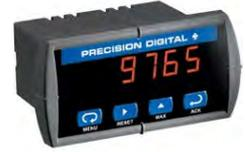
Program and setup using the four front panel pushbuttons or by using the free MeterView™ software. Password protection restricts modification of programmed settings. Units with relay output option have functionalities that include automatic reset only, auto/manual reset, latching/non latching, pump alternation control, on/off time delays from 0 to 199 seconds and fail-safe operation. Adjust the intensity of the display to compensate for various lighting conditions, including direct sunlight.
