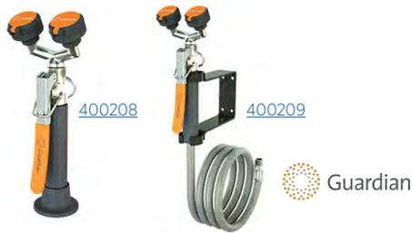
These dual-purpose Eyewash/Drench Hose Units meet the provisions of ANSI Z358.1-2014 as both an eyewash and a drench hose. Locking clip engages when handle is depressed, providing “hands free” operation. Valve stays open until locking ring is released. Alternatively, unit may be removed for use as a drench hose to rinse any part of the user’s eyes, face or body.
