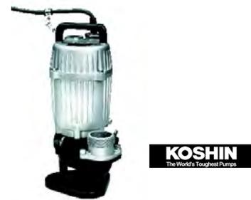
Koshin's Submersible Trash Pump is perfect for municipal, construction and industrial use. Pump only measures 10" in diameter making it great for manhole and vault draining. Water is channeled through the outer wall which cools the motor and provides you with a pump that has maximum endurance.
