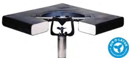
The Aquarian Pro floating aerators have high-velocity propellers that pump a water column creating the best possible oxygen transfer rate. This causes a shearing effect which converts the water column into a highly accelerated spray pattern that obtains oxygen. Mixing and aeration occurs with the simultaneous volume of water being propelled into the atmosphere.
