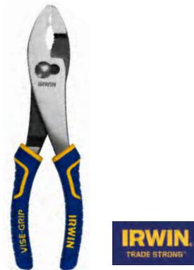
The Vise-Grip Slip Joint Plier has an induction hardened cutting edge that stays sharper longer. The jaws are machined for maximum gripping strength. The plier also has ProTouch™ grips that have molded handles for comfort and create less hand fatigue. All pliers meet or exceed ANSI specification.
