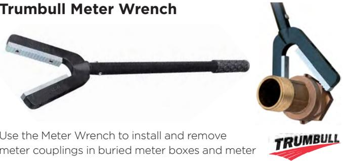
Use the Meter Wrench to install and remove meter couplings in buried meter boxes and meter pits. The 16" handle allows easy access into these confined areas; works with 1/2 to 1-1/2" meter couplings. Special features include resilient grip on handle and replaceable jaws.
