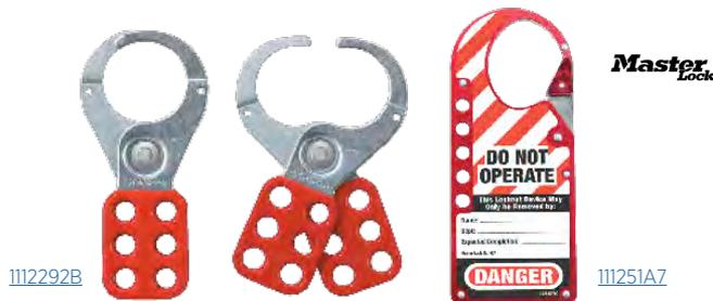
The Lockout Hasps, also known as safety hasps or lockout tagout hasps, are used in lockout/tagout procedures to provide a secure and visible means of isolating and locking out energy sources during maintenance or servicing of machinery or equipment. Hasps hold multiple padlocks, allowing multiple workers to apply their own individual locks, ensuring the equipment remain inoperative until all locks are removed.
