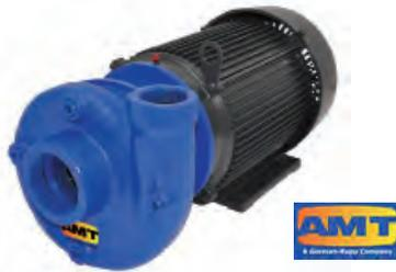
AMT High-Volume Straight Centrifugal Pumps are excellent at handling solids and dirty water in liquid and chemical transfer, heating and cooling, recirculation, booster service and other industrial applications. Semi-open impeller with self-cleaning ability can pump solids up to 1/4" in diameter. Adjust discharge position in 90 degree increments with vent and drain plugs for all positions.
