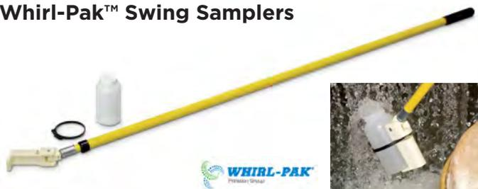
Easily collect samples from a horizontal flowing stream, such as a sewer with the Nasco Swing Samplers. The end of the sampler swings, allowing collection from different angles, including 90 degrees. The 8-ft. adjustable fiberglass pole extends to 12 ft or 24 ft (depending on model) providing a long length for any sampling situation.
