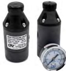
All valves come preset at 50 psi, however they are field adjustable from 10 to 150 psi via the adjustment screw. Robust construction ensures reliability in the rigorous service of municipal and industrial applications. Easily spot check system pressure with the integrated pressure gauge option.
