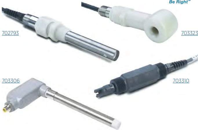
These Conductivity Sensors feature a built-in 1000  $\Omega$  platinum RTD that compensates the measured conductivity for changes in process temperature, resulting in excellent accuracy. Select from contacting and inductive (electrodeless) conductivity sensors.
