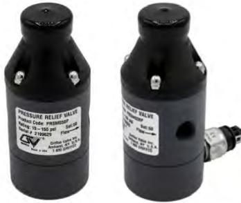
Protect chemical feed systems from over pressure damage caused by defective equipment or a blockage in the chemical feed line using Griffco Pressure Relief Valves. When the preset pressure is exceeded, the diaphragm which is held against the valve seat by an internal spring, is forced up and the chemical flows out the relief port, back to the chemical tank or to the suction side of the pump. Robust construction ensures reliability in the rigorous service of municipal and industrial applications.
