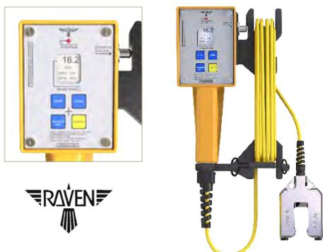
The Raven Sludge Interface Detector is a portable handheld instrument that accurately determines the sludge blanket solid/liquid interface depth in primary tanks, clarifiers, sedimentation basins, lagoons and a wide variety of tanks with settled sludge and solids. The unit is equipped with a strain relieved signal cable with 1-ft increment depth marks and a sensor probe.
