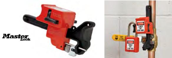
The Seal Tight Ball Valve Lockout is used to immobilize and secure ball valves in either the closed or open position during maintenance, repair or servicing work. The lockout device is designed to clamp tight on the handle to prevent handle movement, preventing the operation or movement of the ball valve to ensure the safety of workers and accidental release of hazardous materials.
