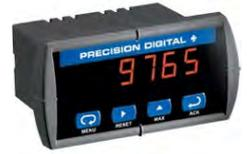
Program and setup using the four front panel pushbuttons or by using the free MeterView™ software. Password protection restricts modification of programmed settings. Units with relay output option have functionalities that include automatic reset only, auto/manual reset, latching/non latching, pump alternation control, on/off time delays from 0 to 199 seconds and fail-safe operation. Adjust the intensity of the display to compensate for various lighting conditions, including direct sunlight.
