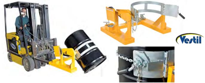
Easily transport and rotate steel drums using a fork truck with the Fork Truck Drum Carrier/Rotator. Rotate drum from the fork truck operator's seat using the included chains. Drum is held securely in place by a durable chain locking system. Drum must be full to rotate at rated capacity. Bung nut wrench is included for opening and closing drums.
