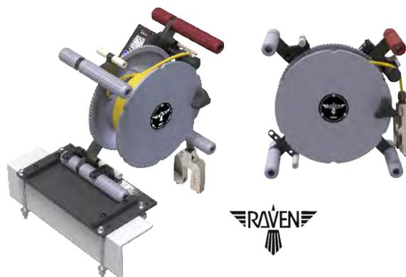
The Raven SID Rotary Portable Sludge Interface Detector is a portable instrument designed specifically to detect the sludge blanket interface and display the interface elevation with a precision depth counter. A robust protective cage, IP67 rated encased electronics, modular components and a solid stainless steel sensor probe ensure reliability and durability.
