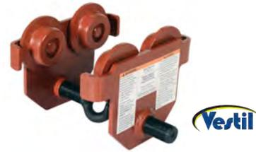
These Push Eye Manual Trolleys quickly install on virtually any S, H, W and M type I-beam. Easily adjust the width of the trolley by rotating the center rod with lifting eye clockwise or counterclockwise. Once the hoist (not included) is attached, the center rod cannot be rotated, preventing the trolley width from accidentally changing during use. Durable solid steel construction with a painted finish and rollers with sealed bearings provide long service life.
