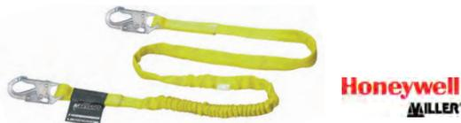
The Manyard shock-absorbing lanyard with locking snaps features a special woven inner core that expands during a fall to reduce fall arrest forces. The heavy-duty tubular outer jacket serves as a back-up web lanyard. A warning flag provides a visual sign if the lanyard was involved in a serious fall so it can be removed from service.
