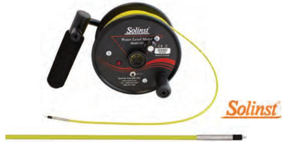
The Model 102M Mini Water Level Meters are designed to measure groundwater levels and are ideal for shallow applications and for accessing very narrow diameters. The included durable P4 probe has no weights and weighs 10 g. When the probe contacts water, the LED light and buzzer are activated. Read the measurement on the cable at the top of the well casing or bore hole to determine the water level.
