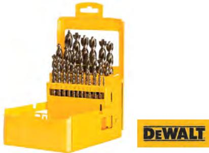
The Pilot Point tips help to keep the drill bit centered on workpiece and provides clean and accurate holes. The no-spin shank eliminates the frustration of bit spinning in the chuck while the tapered web provides greater durability to reduce breaking.
