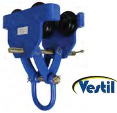
The Quick Install Manual Trolleys adjust to the width of virtually any S, H, W and M type I-beam. Easily adjust the width using a manual screw mechanism which can also be tightened to lock trolley in place. The locking ring prevents the trolley width from accidentally changing during use. Use the lifting eye at the bottom of the trolley to attach a hoist (sold separately). Durable steel construction and rollers with sealed bearings provide longer service life.
