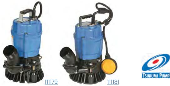
Tsurumi HS-Series Trash Pumps are designed to pump water containing sand, solids and debris with minimal wear and clogging. Compact yet powerful pumps are great for use for sediment removal from small sumps or basins and other industrial/commercial site drainage. Cast iron body and urethane semi vortex impeller provide excellent durability. Select from manual pumps or “Automatic” (Z) pumps that come with integrated float switches.
