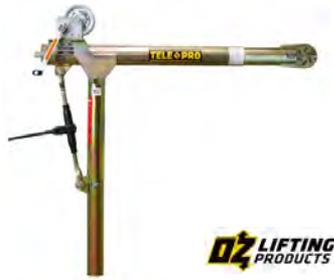
Cranes do not come with base or cable assembly. The cranes use a modular base system to service multiple areas more easily; select from pedestal, socket or wall-mount bases. Cranes also require a cable assembly, choose from either galvanized or stainless steel and with or without a swaged ball. Cable assemblies with a swaged ball can only be used with a manual hand winch, cable assemblies without the swaged ball can be used with either manual hand or electric winches.
