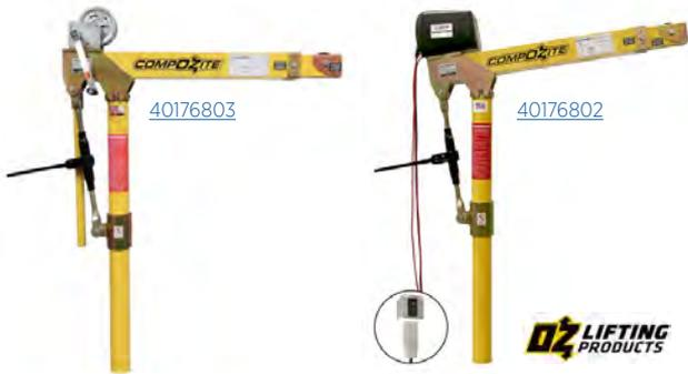
The CompoZite Davit Cranes are made of an advanced composite material, about 40% lighter than steel yet strong enough to lift up to 1200 pounds. Their light weight and ease of assembly and disassembly make them perfect for jobs where the crane has to be moved regularly.
