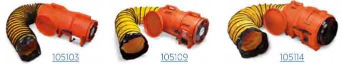
The Plastic Blowers with Canister and Duct Hose provide air circulation, purification and safety in various industrial settings. The quick-connect clipping system allows workers to attach the canister, tools free, to the input side for powerful extraction or output side for ventilation. Retractable, noncollapsible ducts are made of single-ply, PVC-coated, vinyl and polyester.
