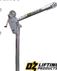
Cranes do not come with base or cable assembly. The cranes use a modular base system to service multiple areas more easily; select from pedestal, socket or wall-mount bases. Cranes also require a cable assembly, choose from either galvanized or stainless steel and with or without a swaged ball. Cable assemblies with a swaged ball can only be used with a manual hand winch, cable assemblies without the swaged ball can be used with either manual hand or electric winches.
